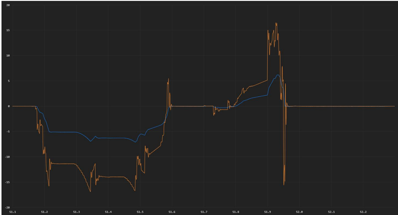
Figure 4: CUNCUN 20, output current in blue, output voltage in orange. X-axis in second, Y-axis in ampere and volt
