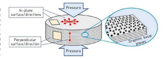
>> The morphology of the components and the manufacturing process lead to a transversely isotropic material: the inplane and perpendicular directions are defined as those parallel and perpendicular to the graphite basal planes.
